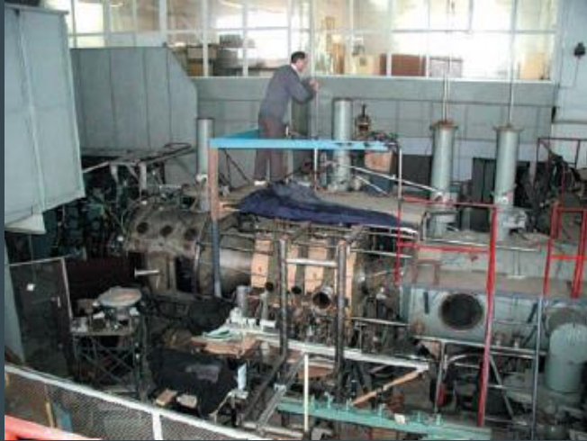
Quasi-stationary plasma accelerator QSPA X-50 (NSC KIPT)
