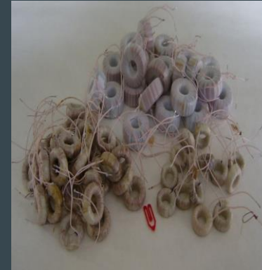
Miniature transformers for high-frequency special-purpose telecommunication control systems
