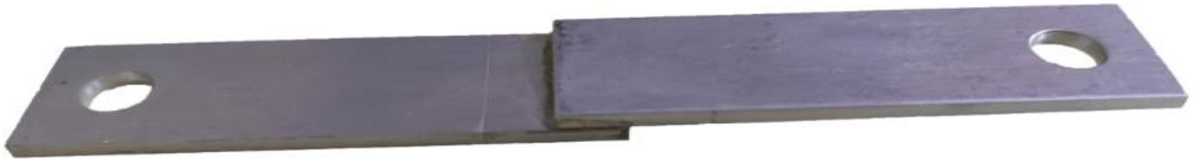
Sample adhesive joint for shear tests.
